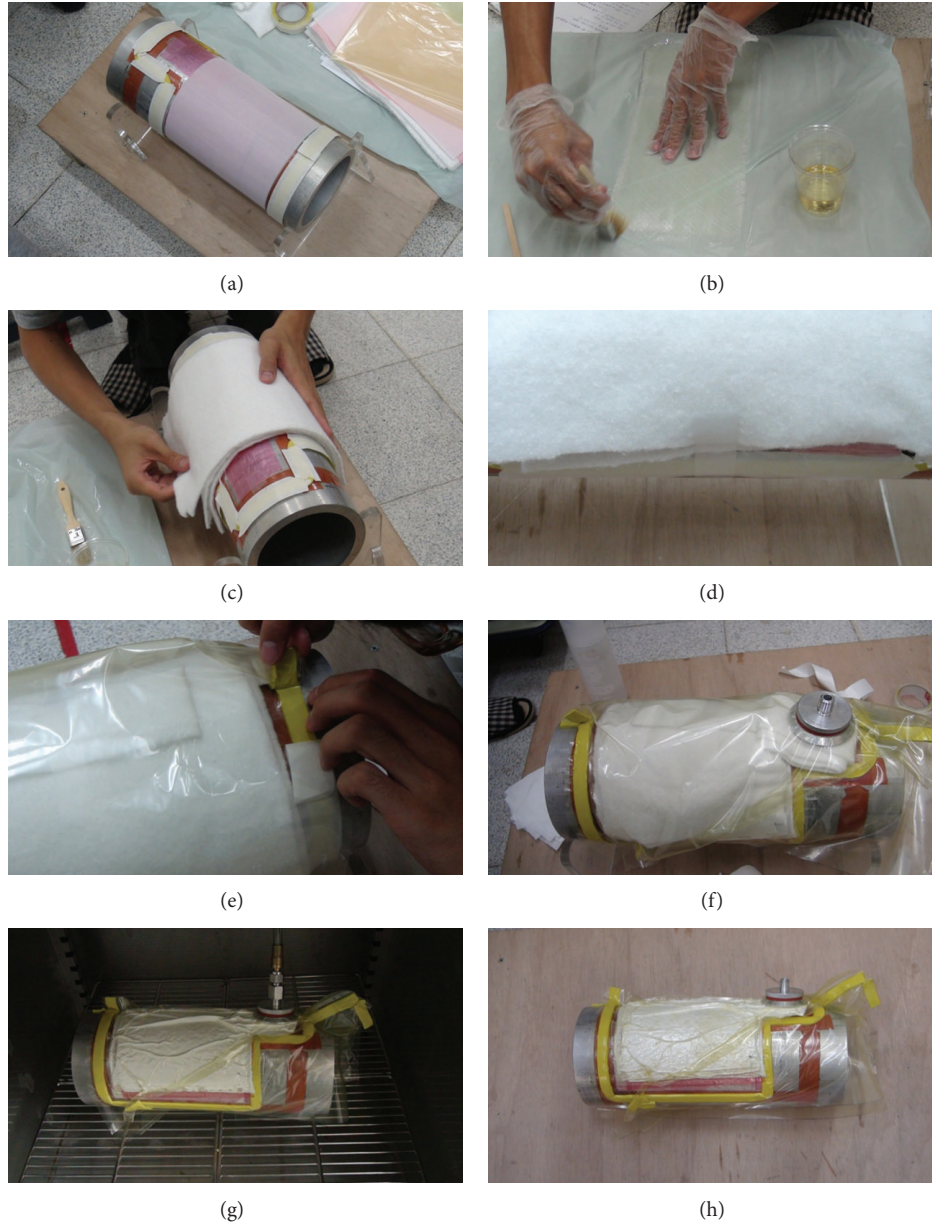
FIGURE 6: Photos of the fabrication process for the fiberglass composites.
